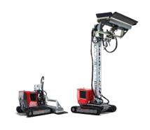
total weight: 2350 kg length: 2,57 - 2,82 m min. width: 1,03 m track width: 1,03 - 1,63 m min. height: 1,3 m\ 1,6 m operating height: 7 m
