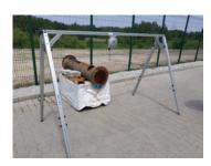
A-FRAME – a steel frame type "A", intended for hanging the FEEDERbox feeder.
