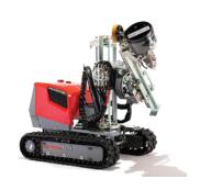
total weight: 1160 kg length: 2,0 m min. width: 0,78 m track width: 0,78 - 1,16 m min. height: 0,99 m operating height: 4 m
