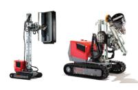
total weight: 1250 kg length: 2,1 - 2,27 m min. width: 0,78 m track width: 0,78 - 1,16 m min. height: 0,99 m operating height: 4 m side reach: 0,95 m
