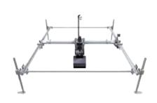
approx. length: 3,3 m approx. width: 2,9 m cutting length: 0 - 2,8 m cutting width: 0 - 2,25 m
