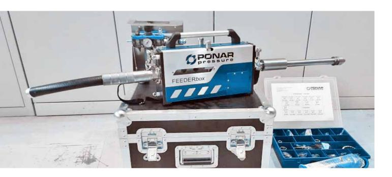
Manipulators are a group of specialized semi-automatic pneumatic elements by PONAR Wadowice, enabling the completion of systems ready for work with the use of flexible high-pressure lances.
