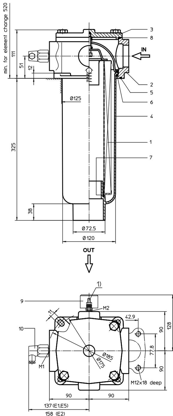
When equipped with one clogging indicator use preferably connection M1.
